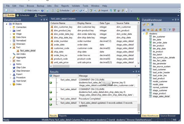
When a staging table is dragged into the list window (middle pane) all fact tables are by default *detail fact tables*. If manually creating a table, then the table type can be selected under the Properties of the fact table.
