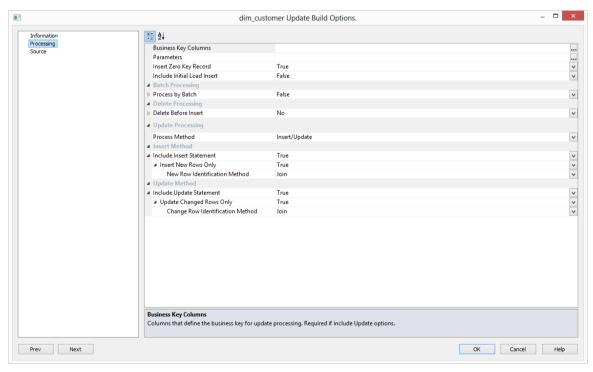
**Business Key Columns:** Columns that define the business key for update processing. This is required for include Update options. The source table from which the dimension is derived would normally have some form of unique constraint applied. In most cases this will be the business key. In the example below **product\_id** is selected as the business key.
