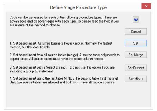
A number of different types of procedure generation are available. Each type is discussed below. There is a checkbox at the bottom of the dialog box. This checkbox will only be present if advanced procedure building features are enabled. This checkbox allows the editing of the 'Where' clause when no table joining is being performed, and hence the 'Where' clause would not be exposed.
