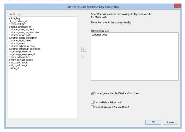
An additional check-box, **Source System supplied Start and End dates** is supplied. This allows for start and end dates to be specified in the source data.
