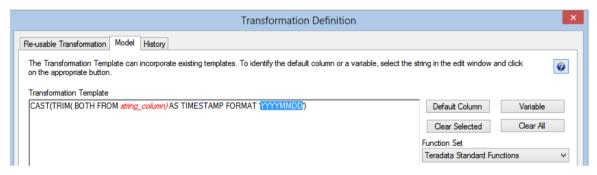
Then highlight the word **format** and click on the **Variable** button. This makes the word **format** a variable than can be substituted when the User Defined Transformation is used.
