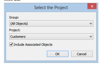
The objects in the diagram will be moved into the selected project. If the **Include Associated Objects** checkbox is selected, this will include all associated procedures, scripts and indexes. The default for this checkbox is on.
