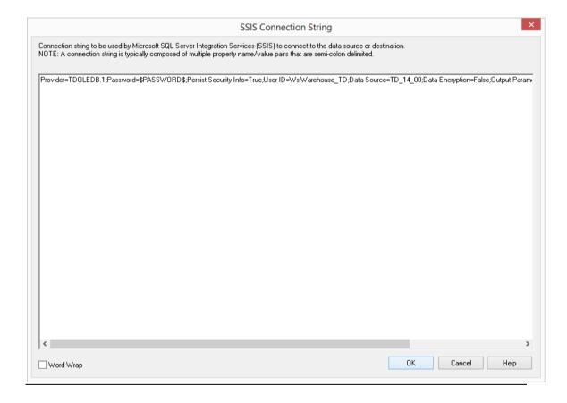
Once the connection is defined then a load table needs to be created to hold data loaded into the data warehouse by dragging a source table or a flat file to create a load table – (see *Loading Data* (on page 189) or *Loading Data from Flat Files using SSIS*). On the load table properties the Load type can be set to *Integration Services load*. This will create and execute a SSIS package at run time to load data into the data warehouse load table.
