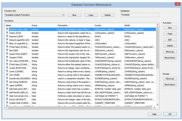
On the right is a group of buttons used to maintain the list of functions in a function set. These buttons are not available for standard function sets.
