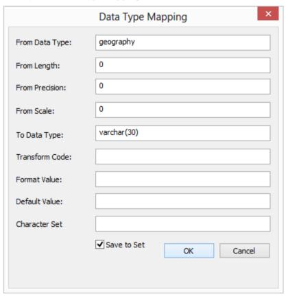
• Clicking the **Save to Set** check-box in the Data Type mapping screen above will save the mapping to the custom set that was used for loading the table.
