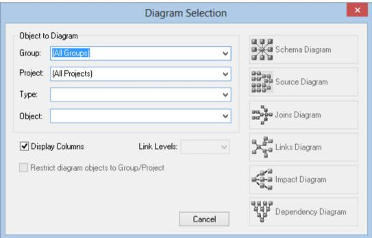
**2** Choose the object to diagram by optionally choosing the **Type** to limit the selection list; and then selecting the **Object**. The diagram type buttons on the right will then become active and you can choose the type of diagram to display.
