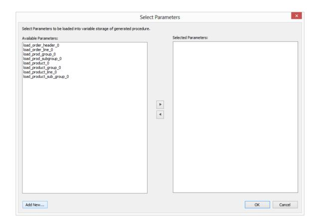
The variables can also be used in column transformations and in the from/where clause for the update procedure. Some databases have a 30 character limit for variable names. WhereScape RED ensures the variables added for any parameters are less than 30 characters long by creating variable names in the form v followed by the first 28 characters of the parameter name.
