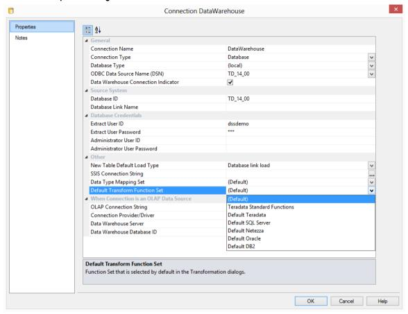
In the Connection Properties dialog, when the **Data Warehouse** check-box is selected, a drop-down list **Default Transform Function Set** is displayed. This is the default set that will be selected in the transformation dialogs above.
