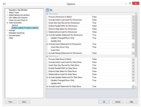
The **Process in Batch** option, when selected, allows users to select a column to drive data processing in a loop based on the distinct ordered values of the selected column.
