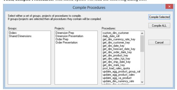
As each procedure is compiled it is displayed in the middle pane of the builder window. If a procedure fails to compile a failure message is displayed along side the procedure name. Procedures that fail to compile will need to be investigated through the procedure editor, as no specific error information is provided by this bulk compiler.
