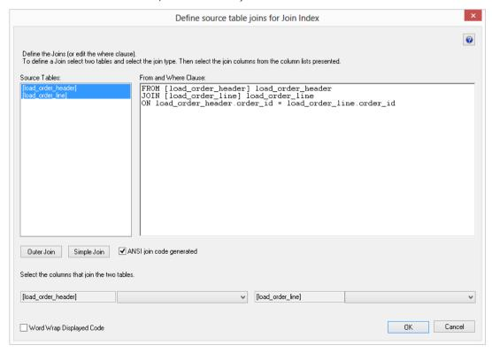
If aggregation is required, proceed to the next section, otherwise remove any checks from the **Sum**, **Count** and **Group by** checkboxes on each column of the join index.
