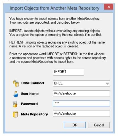
Enter the connection, and a database user name and password that has access to the source metadata repository. Finally, enter the user name of the metadata repository you want to import from. In most situations the 'user name' and 'meta repository' would be the same. However, if you only have read access to a meta repository then it may be necessary to login to the database under a different user name from that of the repository you are trying to import from.
