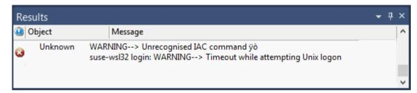
Attempt the connection again, and using the **Window** menu option select the **Telnet** window. This will display the login session, and should provide an insight as to why the connection is not being completed.
