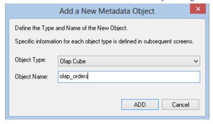
**5** A dialog box will prompt for any OLAP Dimensions that do not already exist that are required for this cube (based on the fact view metadata). Set the dimension name in the **Add a new metadata Object** dialog box and click **ADD**. Repeat this for each dimension as required.
