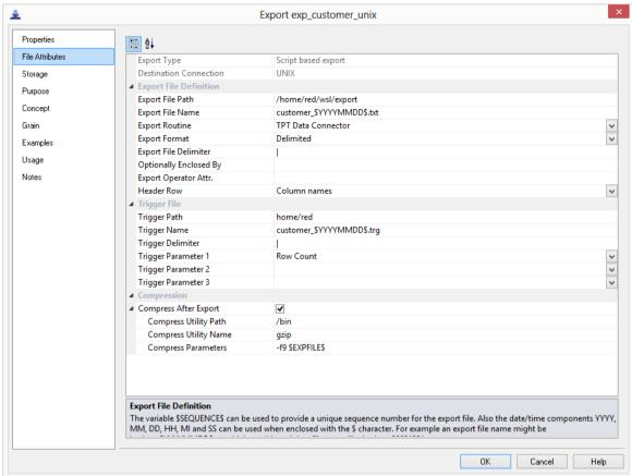
TIP: With all the relevant fields filled in, remember to go back the Properties tab and select (**Build Script**) from the Script Name drop-down menu.
