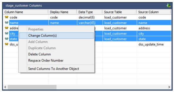
To change a column property, you first need to select the relevant **checkboxes** on the left. Each checkbox, when selected, allows you to change the value for that field in the column properties.
