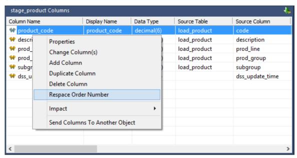
The **Column Order** number for each column will be adjusted so that the column order numbers are evenly spaced.
