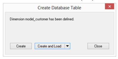
If you are satisfied with the columns that will be used and do not wish to add additional columns you can select the **Create and Load** button. In such an event it would be normal practice to select the **(Build Procedure...)** option from the 'Update Procedure' drop-down list in the previous properties page. If no procedure has been selected then select the **Create** button as no update will occur in any event.
