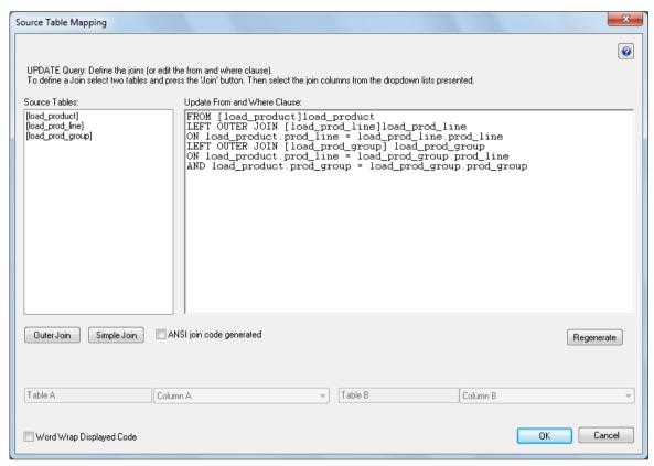
Select two tables in the left box and then click one of the join buttons. The columns for the two tables then appear at the bottom of the dialog and one column is selected from each drop-down list to effect the join between the selected tables. In the example above the load\_product and load\_prod\_group tables are joined by two columns namely prod\_line and group. In such a case two joins are actioned for these two tables, so that both columns can be selected.
