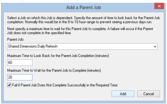
The **Maximum Time to Look Back for the Parent Job Completion** field prevents older iterations of the parent job as being identified as a completion. In our example, we are starting both jobs at 3am, so we don't need to look too far back to ensure that the dimension refresh has run. We have therefore set the look back minutes to 60 to allow for any delays in starting this job.
