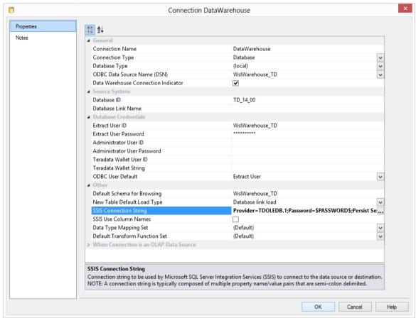
**NOTE:** It is recommended that the password on the SSIS connection string field that is displayed in the connection properties is replaced with the **\$PASSWORD\$** token that is substituted at runtime.
