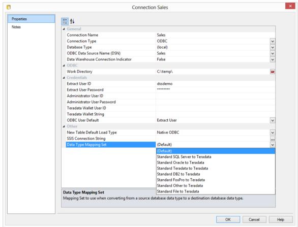
In the Connection Properties dialogs, a drop-down list **Data Type Mapping Set** is displayed.
