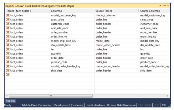
The results of this report are displayed as a list of source tables and columns, the order of the result set determining the immediate lineage. The report includes the following columns:
