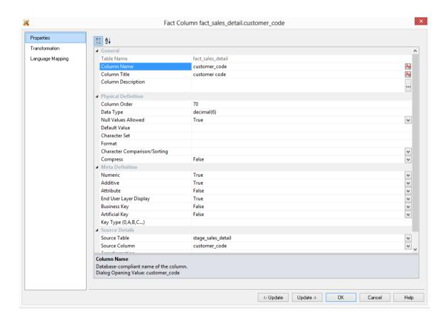
The two special update keys allow you to update the column and step either forward or backward to the next column's properties.
