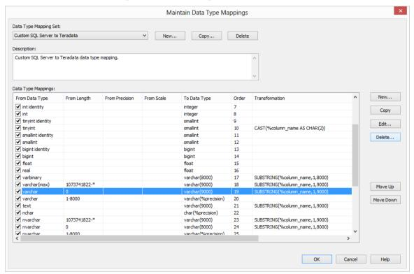
**Note**: The order of the data type mappings is significant as when loading a table, the procedure checks the data type mappings from top to bottom and stops when a data type and its parameters are correctly matched. A blank parameter means that it will match to anything.
