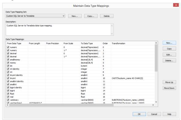
Similarly, you can delete an individual mapping, using the **Delete** button on the right side of the dialog; or you can edit a mapping, using the **Edit** button on the right side of the dialog.
