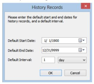
The default interval and interval type should also be chosen. These provide the difference between the end of the previous record and the start of the new record.
