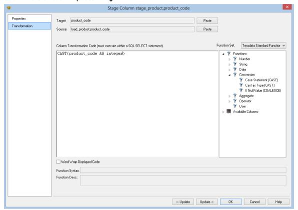
A drop-down list allows the user to select which set of functions are to be displayed in the tree view when creating a transformation on a column of a table.
