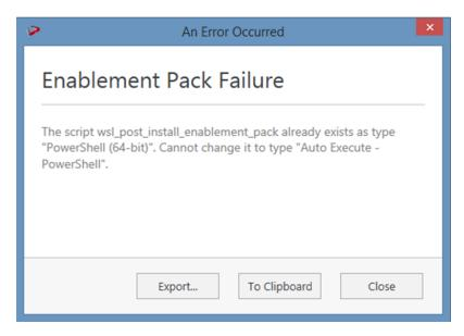
In upgrade of exiting repository if the user gets above error then it means the script type of wsl\_post\_install\_enablement\_pack is set to PowerShell(64-bit) change the script type to Auto Execute-PowerShell before upgrade or manually run the wsl\_post\_install\_enablement\_pack script from host script from RED after upgrade.
